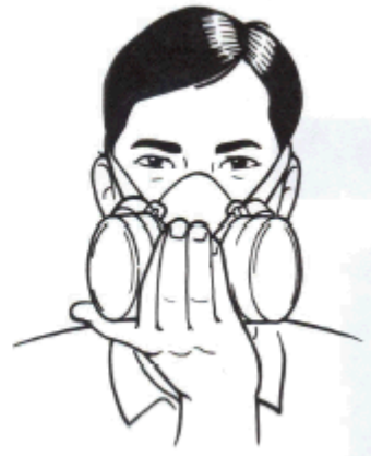
Figure 3: Positive Pressure Check
