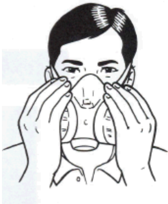
Figure 2: Negative Pressure Check
