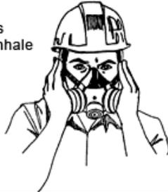
A *negative pressure check* is when the inlet opening of the cartridge is closed off with the palm of your hand, inhale to slightly collapse the face piece, hold breath for 10 seconds. Face piece should remain slightly collapsed with no air leakage – this indicates the seal is working.
