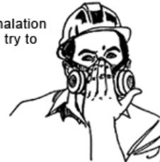
A *positive pressure check* is when the exhalation valve (middle valve by mouth) is covered with palm of hand and as you exhale slight positive pressure is built up inside the face piece. Face piece should fill with air/balloon slightly to indicate the seal is working.
